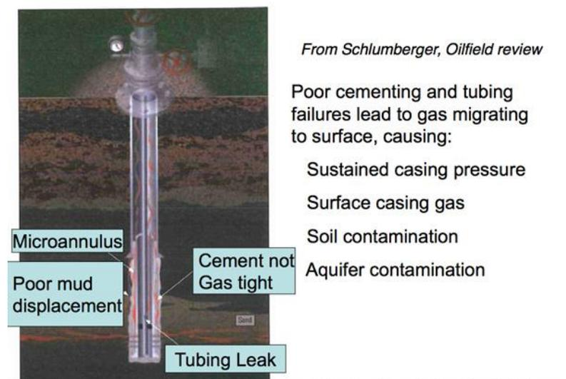
The casings fail for many reasons: failure to ensure gas tight fitting of the metal components; the technical difficulties of ensuring consistent flows and quality in the cement (just about impossible with such long and non-straight boreholes); ground shrinkage around the boreholes; poor mud displacement; and seismicity (natural or induced) destroying the integrity of the cement and distorting the fit of the metal casings.
